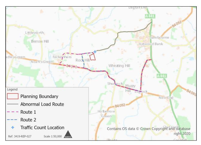
All ALVs will be transported by escort vehicles and temporary road closures would be in place during ALV movements. An Abnormal Load Route Assessment will be undertaken for the anticipated ALV prior to delivery. ALVs are required to approach the site from the east via the ALV route due to constraints on the General Traffic Route.
